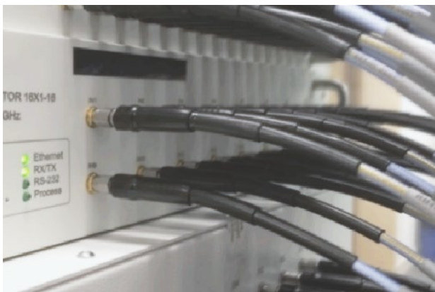
Figure 1: Combining an RF switch matrix or an attenuation array with LAMTA orchestration software can enable software-controlled testing and setup.
